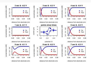
The function plotDiffGrid returns a heatmap showing the concentrations of Ox, Red, and/or Z as a function of time and distance; here we choose to display only Ox and to display only the first 25% of the distance from the electrode surface
